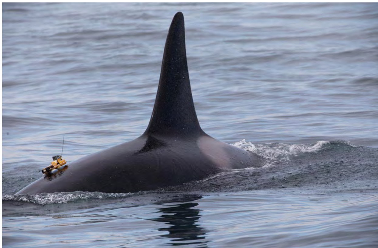
Mixed-DTAG deployed on a sub-adult killer whale, in the optimal placement for effective GPS tracking using the goniometer system.
